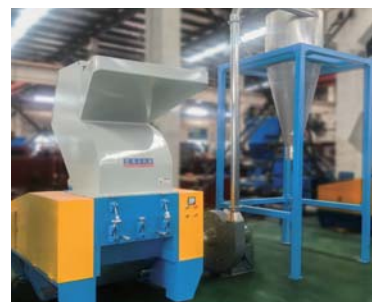
强力破碎机、二次细碎、风机吸料、自动化程度高 Strong crusher, second crush, fan blowing system, high level automation.
