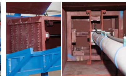
液压推料、结构简单耐用 Hydraulic push, simple structure but durable.
