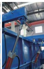
箱盖液压开启、位置检测 The cover is hydraulic opening and position detection.
